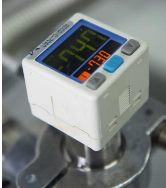
FL( foreline pressure gauge) to Auto on the TMP at safe pressure, Auto off the TMP at dangerous pressure.
