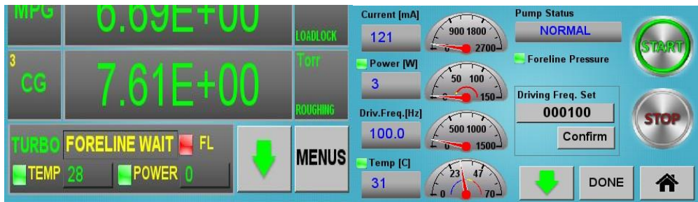
Foreline Pressure Wait (Auto Mode) TMP Freq 100~1350HZ ( 6000~81000) RPM
