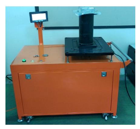
Customized Made, Two Turbo, Two Roughing Pump, Gate Valve
